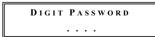
Go on assigning a number included between 0 and 9 to each one of the four figures shown, through the keys used for the selections. Once the setting of the four figures has been achieved, confirm the choice by pressing “1”. In order to get out of this function without saving, press “2”.
