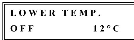
By pressing the key “3”, the display will show ON and temperature will be viewed. In order to get out of the programming mode, press the key “7” and check the result.
